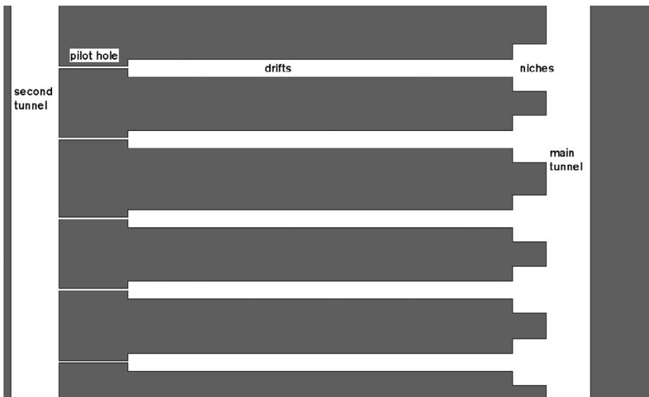
**Figure 9-1.** Schematic illustration of a double tunnel system, drifts are reamed between two tunnels, ~40 m rock is left in the end and only the pilot hole has to be plugged at that side.
