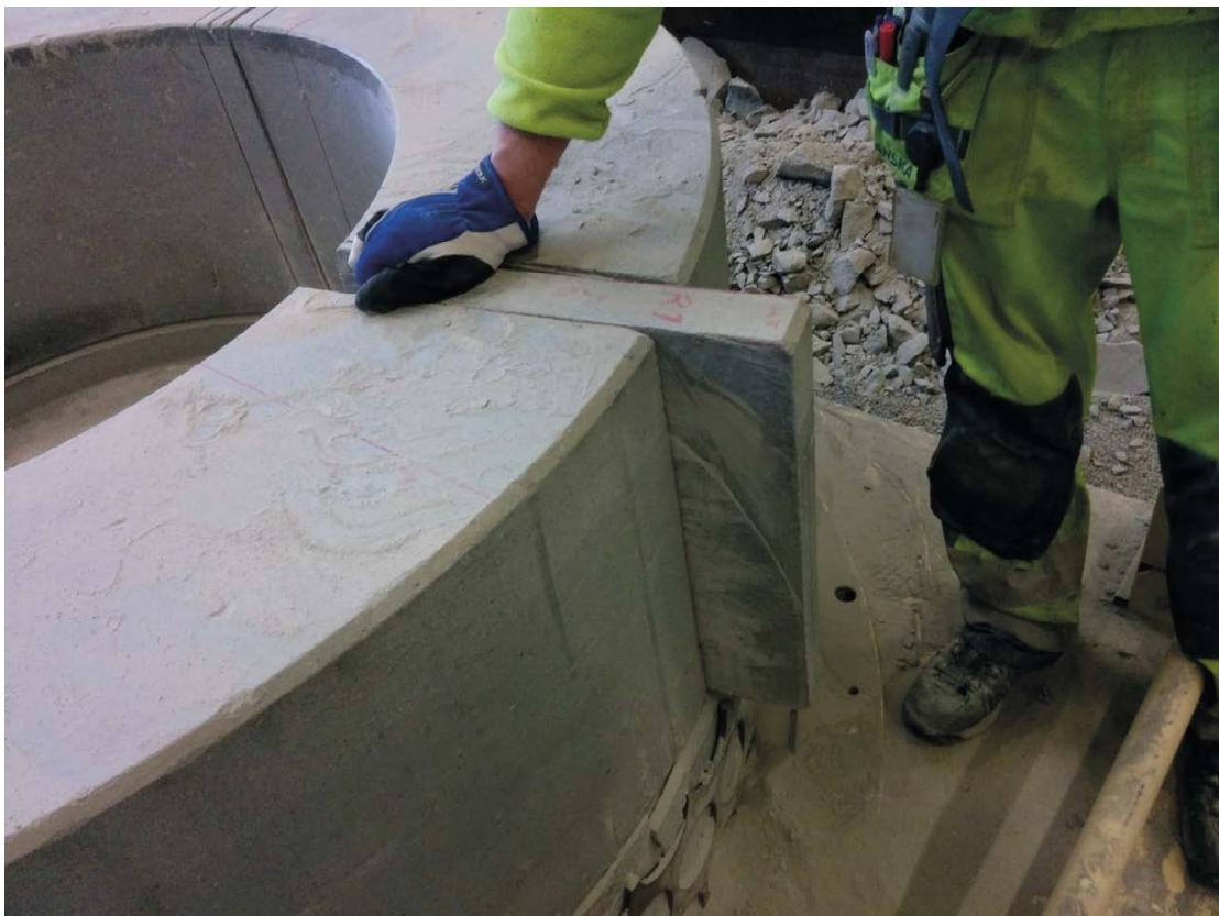
**Figure 5-22.** Taking samples from the buffer rings.
